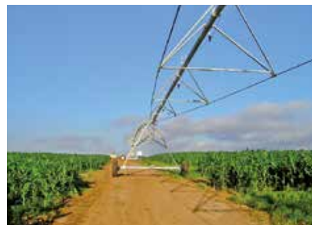
Easy towing thanks to the easy rotation of the drive tower wheels
