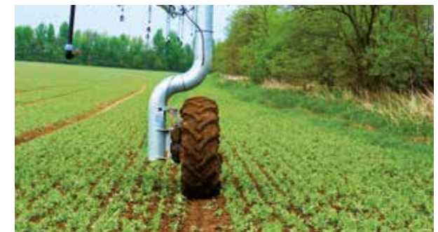
Precise control via GPS control system. Drive wheels are rotatable.
