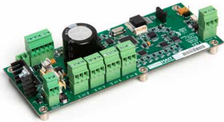
4 WAY LATCHING SOLENOID (12VDC) CONTROL BOARD WITH ONE INPUT, MULTI CHANNEL DATA LOGGER - 4 way 12VDC solenoid control board
