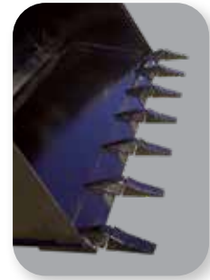
Multi-purpose bucket with ground engaging teeth fitted
